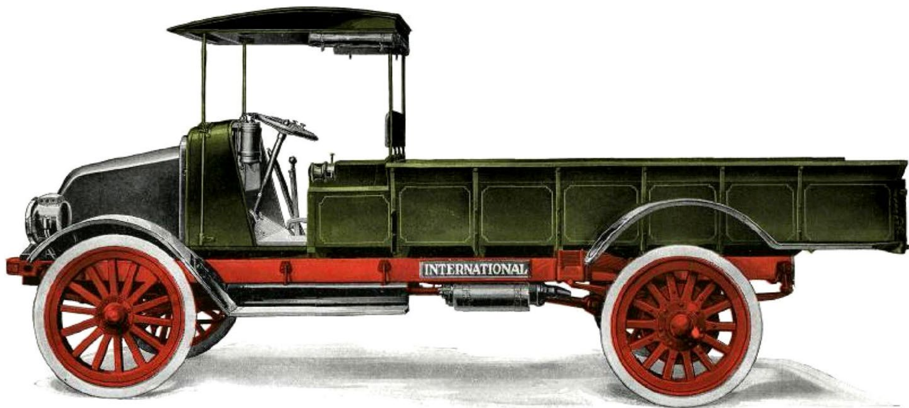
Illust. 1—Model G, International Motor Truck—capacity 2 tons. Equipped with regular express body and cab top.
