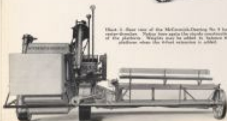
FIG. 4. Right side of McCormick-Deering No. 9 harvester-thresher with steel chaffer removed to better show the construction of the machine. Notice the strong loading platform and the extra steel for the straw roller.
